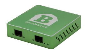
BarnMini-02 is equipped with 2x SFP cage with interconnection TX to RX and RX to TX. The functionality is dependant of the kind of SFPs inserted. The examples only show a selection of typical setups.
